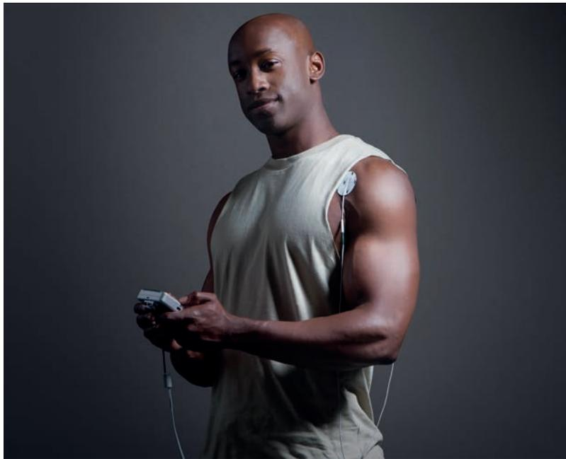
The technology uses electrode pads and ear clips to transmit microcurrents
