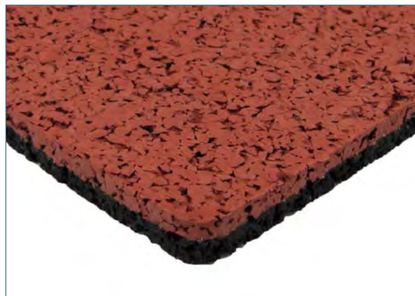
everroll® kombi – typically consists of a 4 mm thick elastic layer and a 4 mm thick EPDM top layer.
