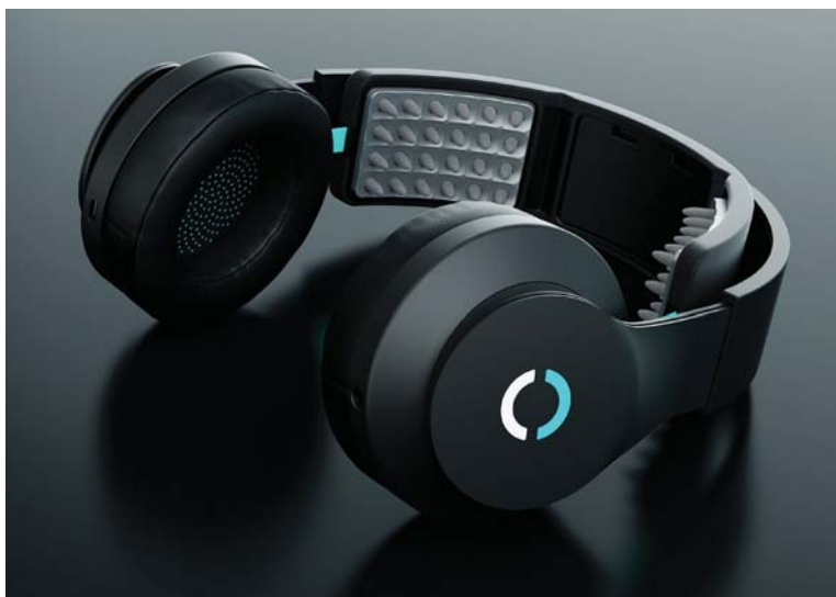
Halo uses spikes to deliver electrical waves to the athlete’s brain
