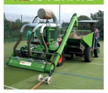
The unique REPLAY REJUVENATION° air extraction process will restore contaminated and compacted carpet to a clean 'as new' condition - extending the life of the facility at a much lower cost than replacement.
