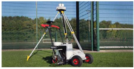
The system allows the immediate and accurate marking of outdoor sportsfields in one go
